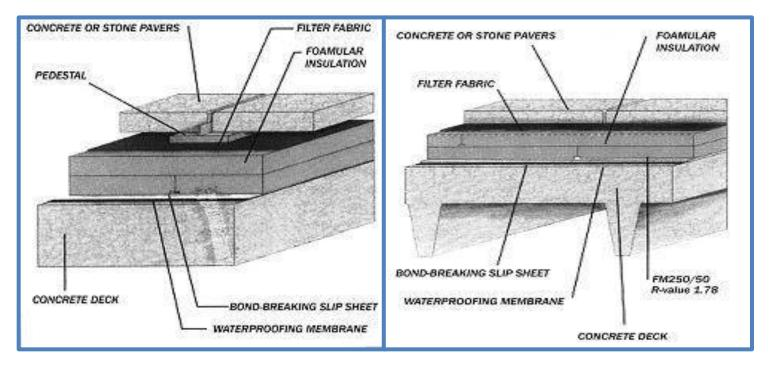
Lightweight yet tough and durable Foamular metric boards are easy to hoist, handle and Install. The boards add little weight to the overall roof structure while providing long term protection to the waterproofing membrane. Board size is 2450 x 600 in thicknesses from 25 to 100mm
