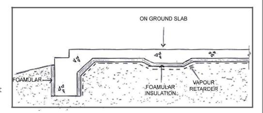
3. For **maximum performance** Foamular is laid against slab edge, over flat areas and into trenches prior to concrete pour as below.
