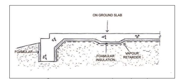
The Foamular is laid directly over the slab area with supports and reinforcement placed on the Foamular.
