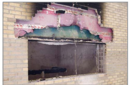
Figure 5: FOAMULAR® showing limited damage above the test window with brick veneer stripped away after the fire test
