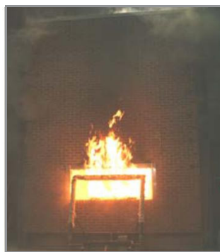
Figure 4: Fire emitting from the test window
